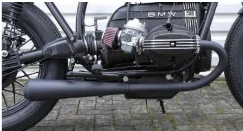
Mounting shows the right side, left side must be mounted accordingly!
