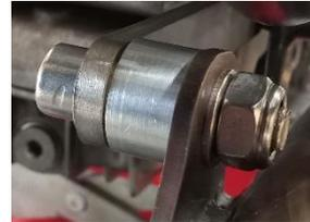
11. Align the exhaust system and tighten all screws connections, starting from the outlet, of the exhaust system from front to back, so everything is in line
